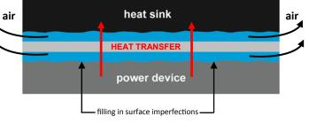
Note: during initial phase-change, it is recommended to re-check your torque settings if device utilizes a screw mounting system. Applying additional torque during initial phase change will thin the material bond line slightly leading to improved thermal performance.
