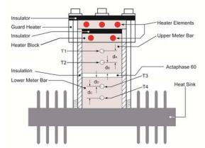
$T_{\rm A}$  = T2 - d\_{\rm B}/ d\_{\rm A}(T1 - T2) = Temperature of upper meter bar surface in contact with Actaphase 60 Pad
