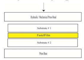
General setup for bonding and sealing heads of mechanical fasteners / plugs / screws. Apply heat using a curing oven, heat tunnel, heat gun, hydraulic or mechanical press.
